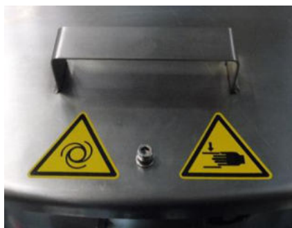
Figure 6 Handle & locking screw
