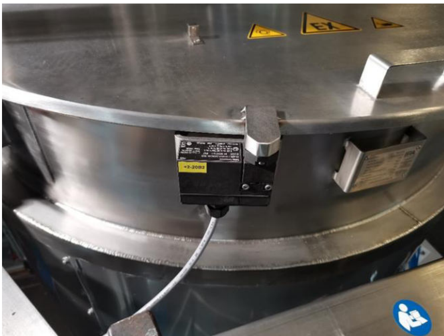
Figure 15 Container lid guard locking
